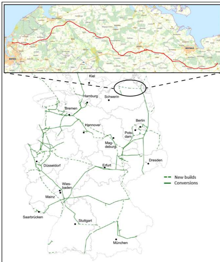
Figure 3.23: National approved Hydrogen Core Network (HCN) of over 9000 km length. The green solid lines (~56%) show existing pipeline segments which will be converted to transport H 2 while the green dashed lines (44%) show the pipelines to be built in the future.
