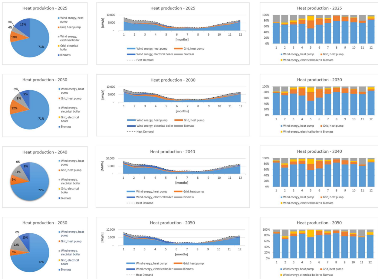
Figure 3.17: Estimated heat production from wind energy using a 6 MW heat pump and a 6 MW electric boiler. The rest of the heat demand is reached using electricity from the grid and biomass
