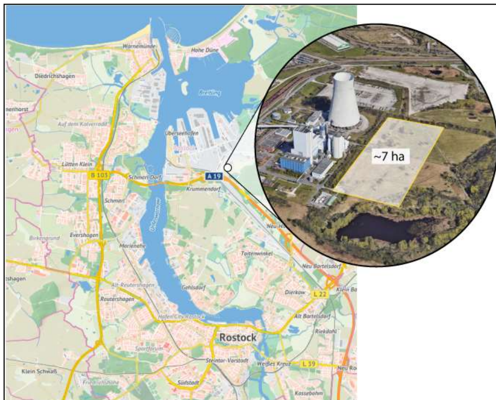
Figure 3.21: Planned location of the electrolyser at the Rostock Overseas port next to the coal-fired power plant. The 7-hectare facility will be in close proximity to already existing infrastructure (pipelines, roads, etc.).
