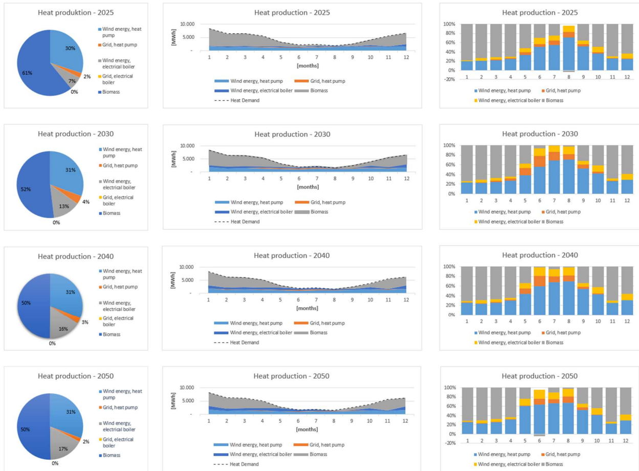
Figure 3.18: Estimated heat production from wind energy using 3 MW heat pump and 4 MW electric boiler. The rest of the heat demand is reached using electricity from the grid and biomass.
